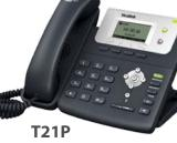
10/100Mb ethernet 132 x 64 pixel graphic LCD 2 SIP accounts
